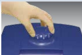
To prevent reagents from evaporating, the height of the hot lid is adjustable to suit all kinds of tubes.
