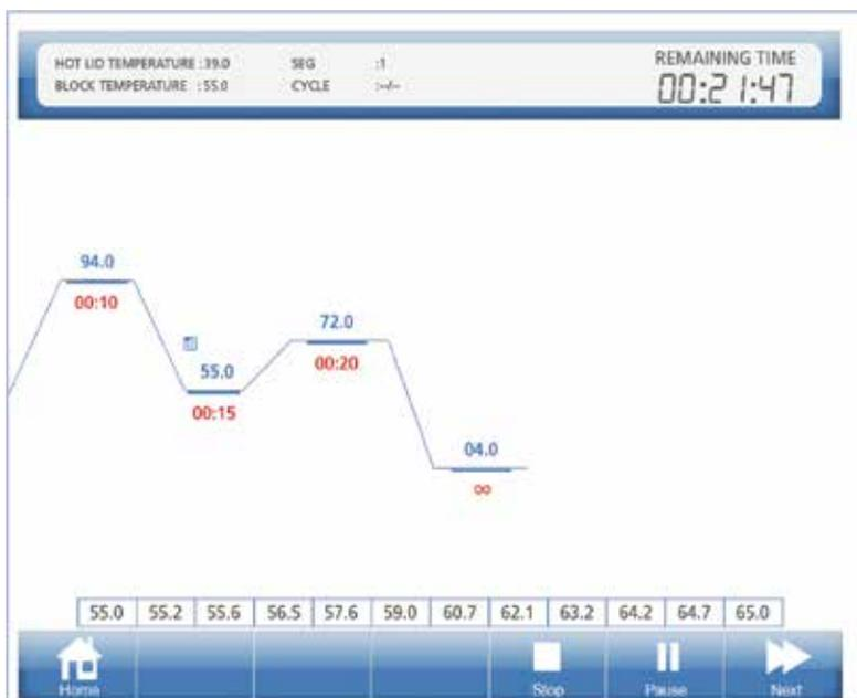
The purpose of the gradient function is to determine the optimal annealing temperature. It's particularly useful when testing suitable annealing temperatures for primers.
